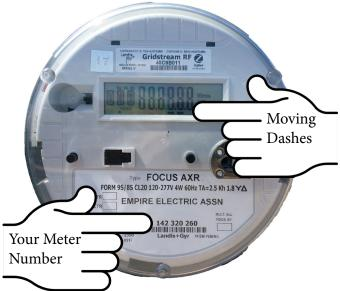
The first screen is an LCD display test that lights up all information on the display to ensure readings display properly. The 2 dashes under the numbers will move from left to right and their speed indicates how much power is being used. The faster they move, the more power is going through the meter.
