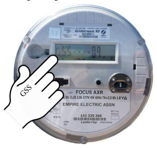
GSS: This is a diagnostic screen and displays codes for faults and communication strength.
