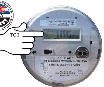
**TOT:** This screen displays the total kilowatt hours (kWh) that have been used by the meter since it was installed.
