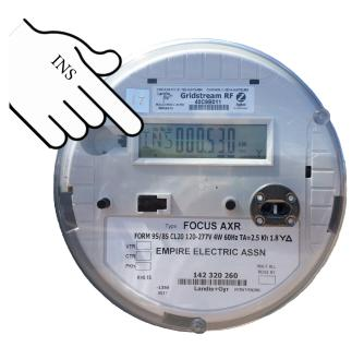
INS: This is the instantaneous Demand in kW and is the amount of power flowing through the meter in real time.
